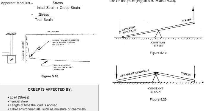
Since the stress is kept constant and the weight or load is not changed or removed, the equation becomes:
