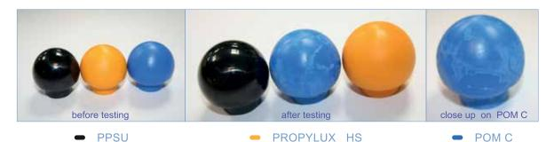
Effects of Disinfecting ProcessPOM CPPSUPROPYLUX® HSDiscoloration/MottlingModerateNoneNoneStress CrackingSlightNoneNoneEtchingSevereNoneNoneOutgassingSevereNoneNone
