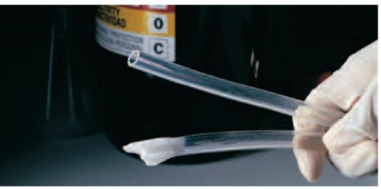
After being immersed in aggressive MEK for 16 hours (plus 4 hours drying time), Tygon® 2075 Ultra Chemical Resistant Tubing is still clear and flexible while PVC tubing is completely degraded and rendered useless.
